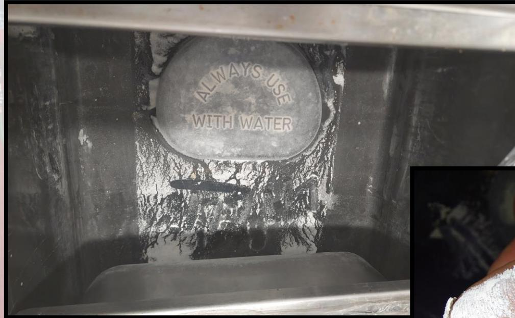
Loose scale powder collects in the bottom and rinses out easily.
